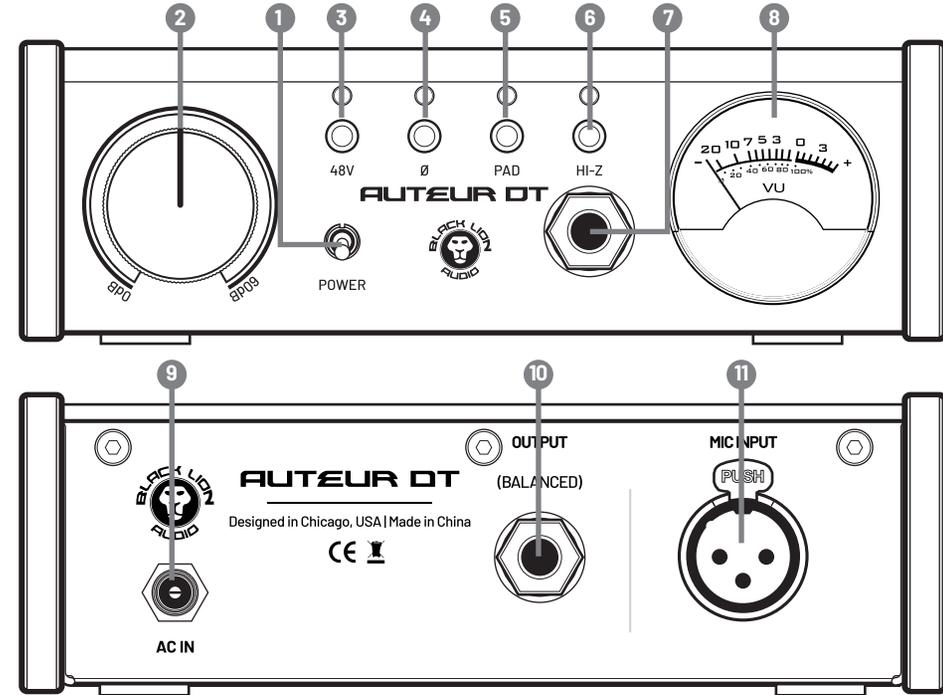
1. **Power:** Flip switch up to turn preamp on, flip switch down to turn preamp off.
