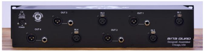
There are XLR inputs for each channel, and both XLR and TRS jack output sockets, which are wired in parallel and will make it easy to plumb this into any home or professional setup. Power is delivered to the B173 Quad via an external line-lump power supply.
