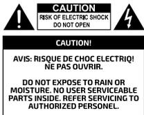
The lightning flash with an arrow-head symbol within an equilateral triangle is intended to alert the user to the presence of uninsulated "dangerous voltage" within the product's enclosure that may be of sufficient magnitude to constitute a risk of electric shock
