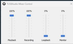
For example: When the loopback fader is increased, audio from your computer's main outputs (Monitor Out L/R) will be sent directly to Application Recording channels 1/2 (Line In 1/2). This is useful for when you would like to record or stream audio playing from your desktop such as sound from videos or music players.
