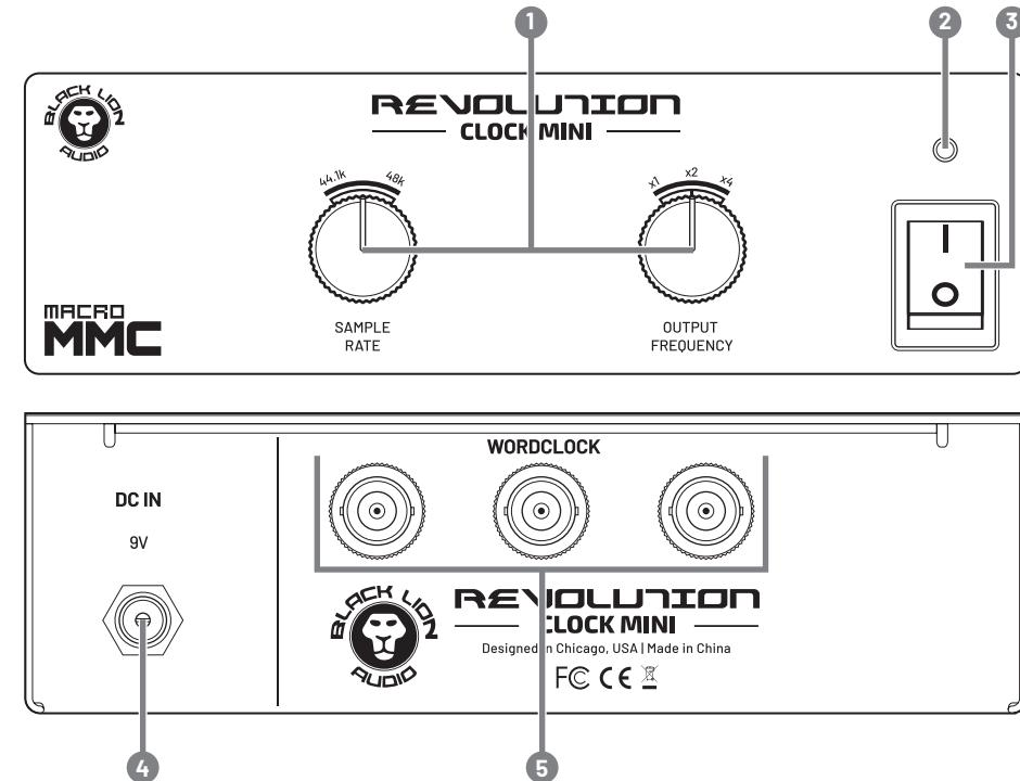
**1. Sample rate selectors:** Use SAMPLE RATE in conjunction with OUTPUT FREQUENCY to choose the desired sample rate. Choose from 44.1kHz-192 kHz.
